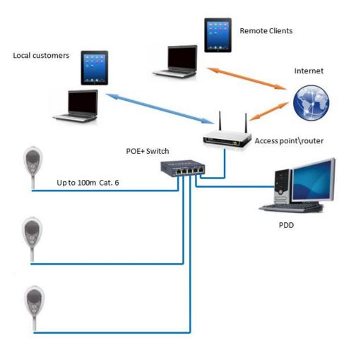
Below is a typical installation structure in the case of a Wi-Fi network:
