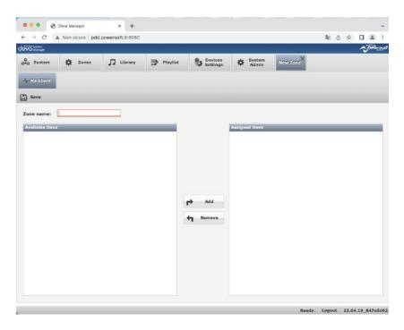
As for the playlists, after entering the name of the new zone, Devas installed in that area, chosen among those not yet associated with any zone, must be added from the left pane to the right one with the usual **Add** button. To remove a Deva from the zone, just select it from the right pane by clicking on the **Remove** button. At the end, click Save and the new zone will appear in the grid.
