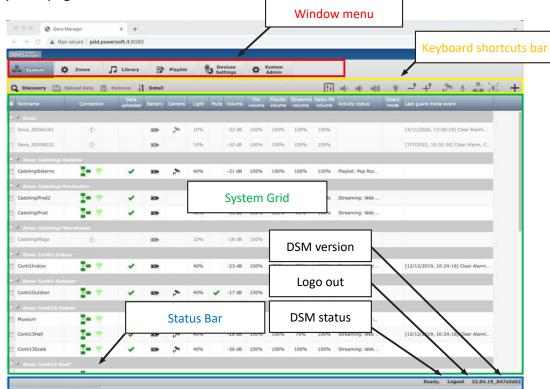
The page consists of: a window menu (indicated by the red rectangle), a hot key bar (indicated by the yellow rectangle), a system grid (indicated by the green rectangle) and a status bar (indicated by the blue rectangle) that shows the status of the "Ready" system, a "Logout" button to log out and the DSM version. Focusing on the "System" page. Below is an explanation of the purpose of the hotkeys.
