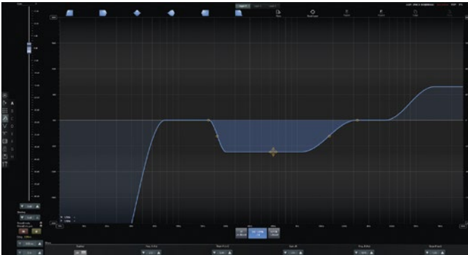
ArmoniaPlus User EQ with raised-cosine filters; three independent layers are available per channel (Fig. 2)
