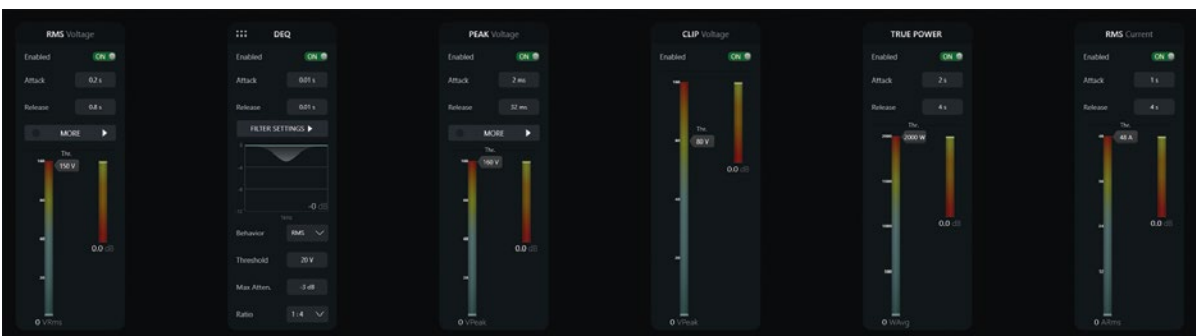
Detailed limiter functions with RMS, peak and clip limiters as well as a current and true power limiter. In addition, a dynamic EQ is also included; the filter's gain is controlled by the signal level (Fig. 4)
