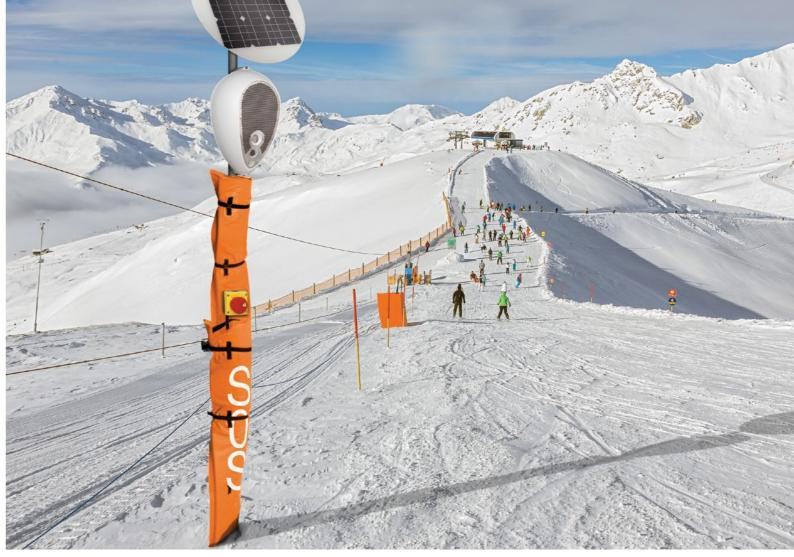
**DEVA** can be installed at the edges of the ski slope, effectively becoming an SOS point. Thanks to the microphone and the camera the unit allows skiers to talk in real time with the control room to request a rescue intervention or to communicate possible dangers on the ski slopes.
