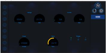
The CPU window offers Voltage, Current, Power, Temperature, and Phase Monitoring at a glance.
