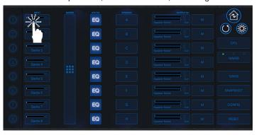
Within the Input window, by tapping on the AES 3 button, it is possible to monitor the AES 3 Signal Status.
