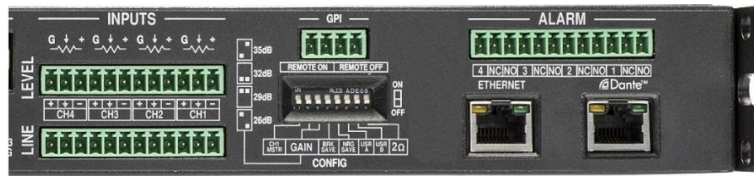
Figure 13 – Canali GPIO Section
