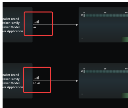
Figure 8 – +5V applied to GPI1 has muted channel 1, nothing applied to GPI2 means that channel 2 gain is unaffected.
