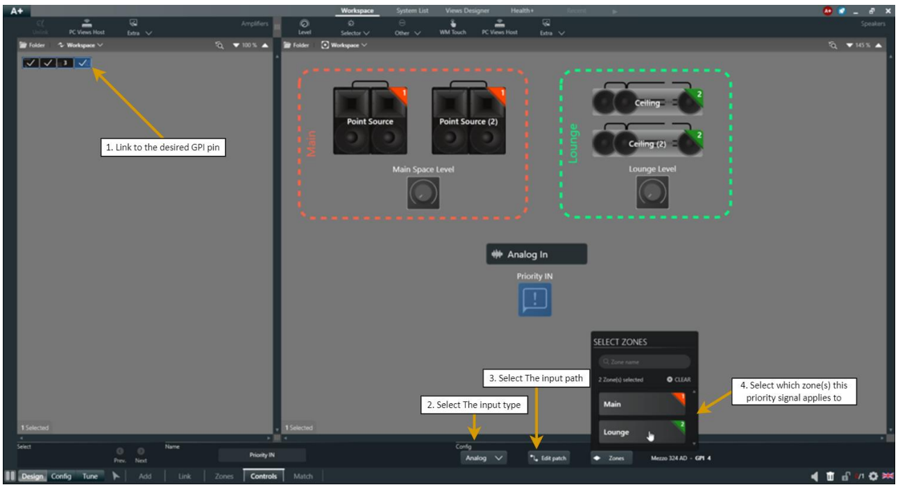
Figure 43 – Adding a GPI triggered priority input (part 2 – linking the object to the GPI)
