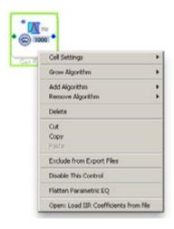
Right-click on a block to bring up the block's pop-up menu. This menu includes items for control Settings, Add/Remove Algorithm, Grow/Reduce Algorithm, Changing IC, and Cut/Copy/Paste editing.
