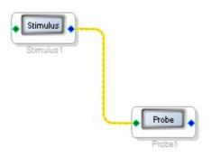
In order to display the response of two or more signals (corresponding to different Stimulus Blocks) in the same Simulation Probe window, right-click on the "Simulation Probe", and select add pins.
