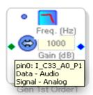
Hover over a block's pin with the cursor to display the pin's tooltip which includes the pin number, unique name, and signal data type.
