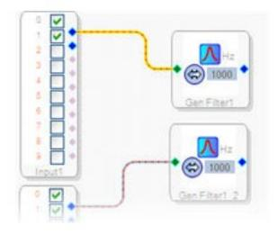
Wires are colored according to their associated DSP processor. The input and output pins of the wire must be associated with the same DSP or you will not be able to create a wire between the pins. Projects with more than one processor IC will have distinct colors for each IC.
