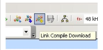
Once the project has been downloaded to the DSP, the system will be responsive to any real-time changes made to controls (sliders, knobs, etc.) in the schematic workspace, allowing to adjust parameters in real time, perform A/B realtime comparison between different projects, and store the preset into the DSP.
