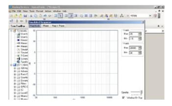
Magnitude and phase response can be displayed both individually or in the same graph by clicking on the tabs located on the top of the window.
