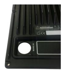
Replace the female PowerCon connector with LiteMod4HC Mains Cable (CB000727) and screw it to the Heathsink. Once CB000727 is in place, connect it to PL1 on LiteMod4HC. Fasten the Earth cable to the LiteMod4HC Grounding screw with the M4 bolt included.
