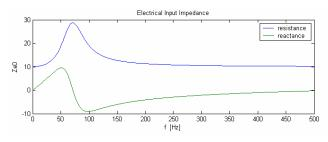
FIGURE 4: Example of frequency response of a typical Speaker Circuit
