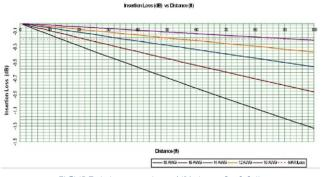
FIGURE 6: Insertion Loss (dB), best if <0.2db
