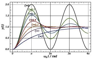
FIGURE 1: Second order system, various damping behaviors
