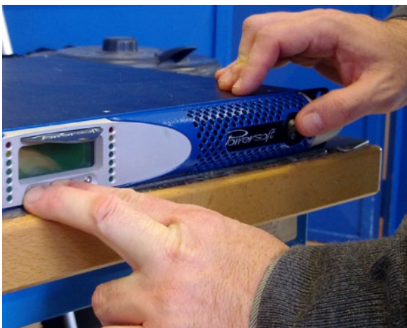
FIGURE 2: Switch on while pressing two left-hand buttons; keep them pressed until yellow LEDs start blinking.
