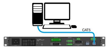
The PC's IP Address must be set to static via the Internet Protocol (TCP/IP) Proprieties.
