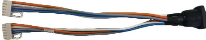
**Warning: Speakon pair going to PL2001 (OUT2) has reversed polarity: negative on 2+ and positive on 2-.
