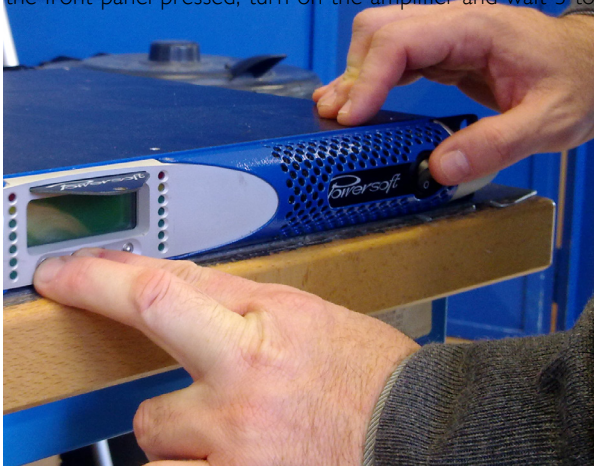
FIGURE 2: Switch on while pressing two left-hand buttons; keep them pressed until yellow LEDs start blinking.
