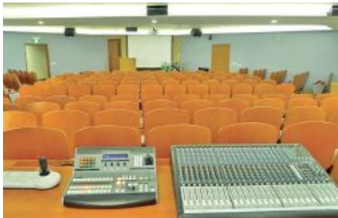
A Mackie Onyx 24-4 console, Sony camera remote control unit and Blackmagic Atem1 switcher are used in the second Sanctuary
