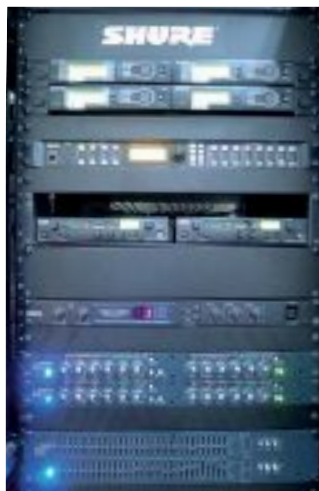
A rack of analogue processors, limiters, reverbs and EQ installed in the rear control room
