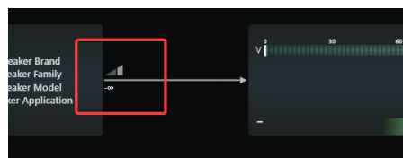
Figure 39 – +5V applied to the Level input has muted the output.
