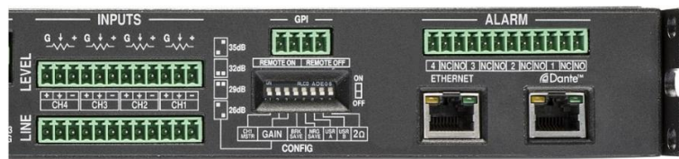
Figure 19 – Canali GPIO Section
