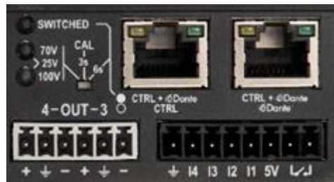
Figure 9 – Mezzo 602 AD GPIO Section
