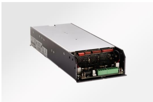
Figure 27 - IPAL Amplifier Module with DSP inside
